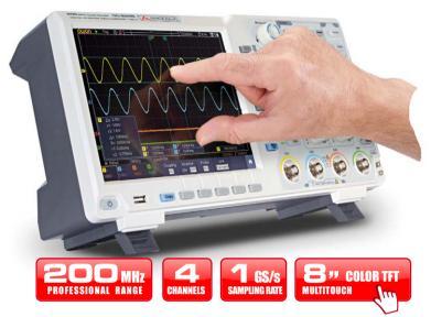
**PROMAX OD-624B** is a digital storage oscilloscope featuring up to 200 MHz of bandwidth and up to 1 GS/s real time sample rate. This professional range digital oscilloscope features a 8" multitouch screen.
