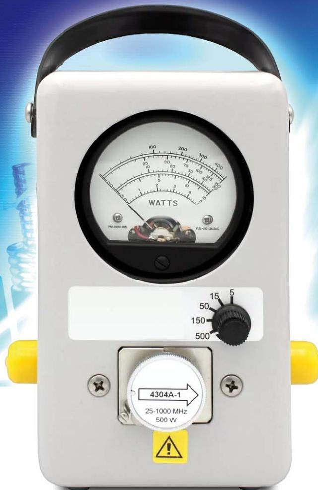
The PROMAX **IC-002B** directional wattmeter measures RF power and load match in 50 Ω coaxial transmission lines. It can be used with CW, AM, FM, and TV modulations, with pulse modulation being excluded.
