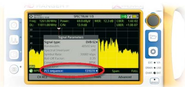
**HD RANGER+** are compatible with this type of signals. In order to certify the proper reception of the digital service, the user only needs to specify the PLS sequence to work with, so the analyser can decode the image.
