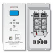
Control module with a dual redundant power supply of 300 W and two inputs for 1 or 2 different electricity suppliers. Each power module is individually removable and hot-swappable. It works when either one of the electricity suppliers or one power module fails. In this case the second power module acts immediately without affecting the TV distribution system.
