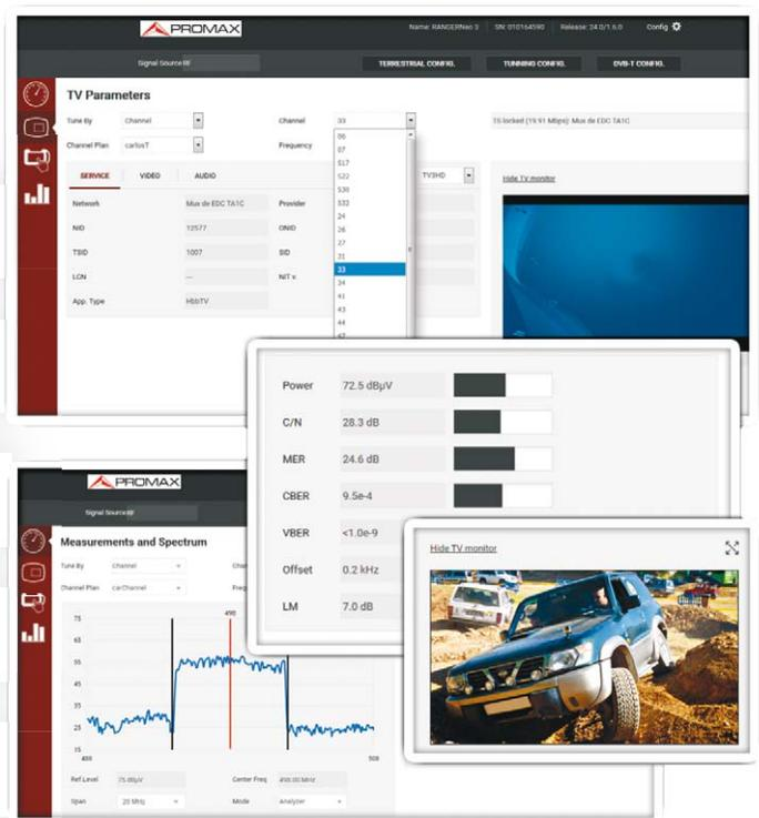
The screenshot displays the PROMAX webControl interface. The top section shows 'TV Parameters' with fields for Channel, Channel Plan, Network, and App. Type. Below this is a table of parameters including NID, TSD, LCN, and App. Type. The middle section shows 'Measurements and Spectrum' with a spectrum plot and various measurement parameters like Power, C/N, MER, CBBER, VBER, Offset, and LM. The bottom right section shows a video player displaying a car.
