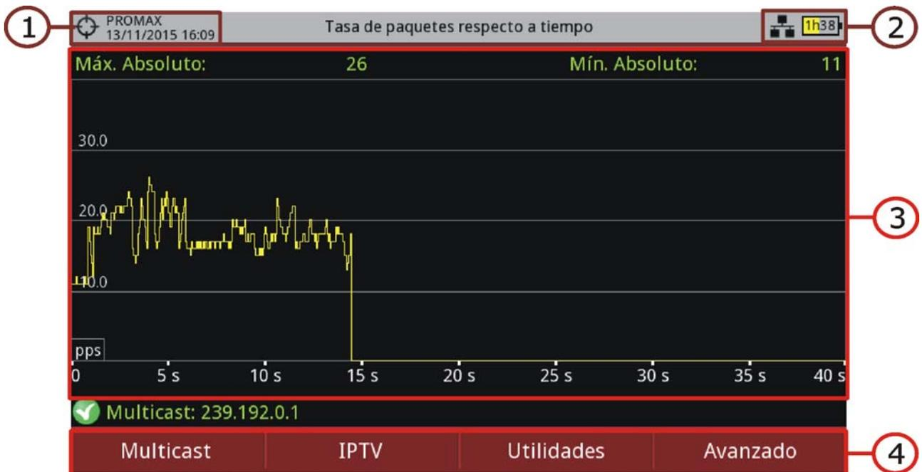
Figure 134. Packet Rate Over Time
