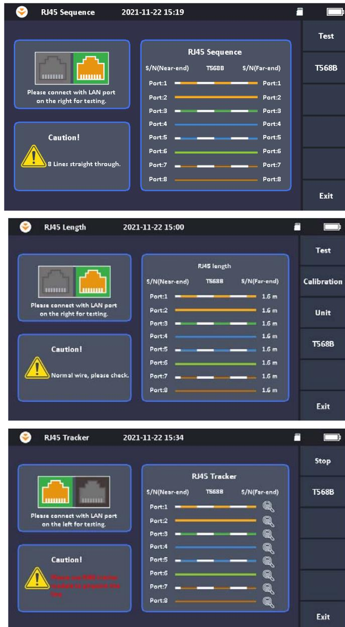
Plug network cable into the LAN1 port to track the cable with tool "Wire Tracker Receiver" together provided.
