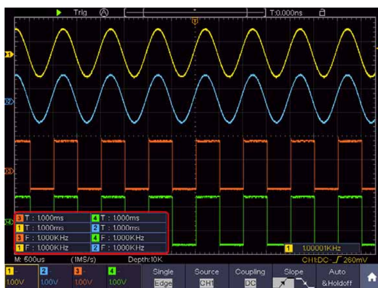
Figure 0-1 Measure period and frequency value for a given signal
