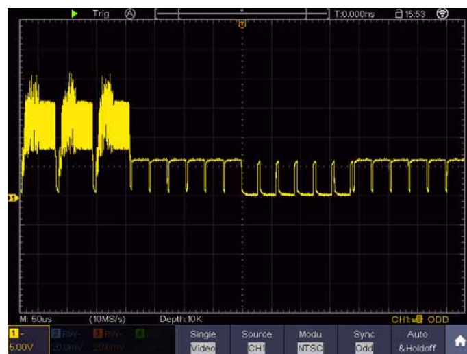
Figure 0-7 Waveform Captured from Video Field Trigger
