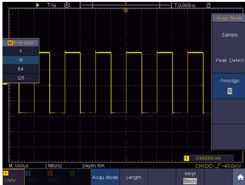
Figure 0-5 Reduce Noise level by using Average function
