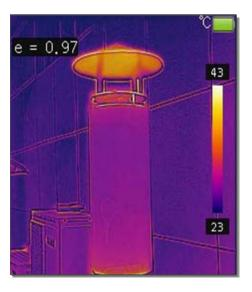
Press and hold the Freeze/Back button to make calibration if the imaging has bad quality or retention.
