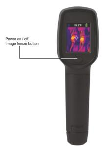
Note: After turning off the device, it is recommended to wait at least ten seconds before next start-up to ensure the safety of the camera.
