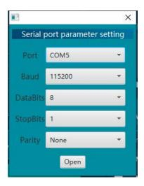
2. Set the serial port number, click the drop-down list, and select a COM number corresponding to the COM number of "USB-SERIAL CH340". Other parameters are the default values.
