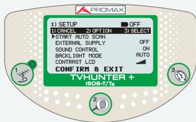
At the **DETECTION** screen, press and hold until appears the configuration menu.
