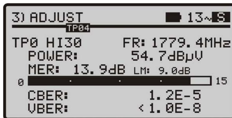
Figure 14.- DVB-S measurements with VBER.
