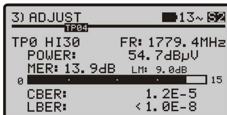
Figure 15.- DVB-S2 measurements with LBER.
