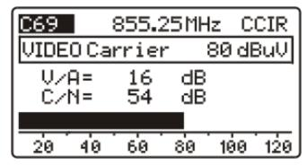
Figure 15. V/A and C/N Level measurement.
