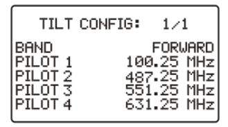
**Figure 47**. TILT configuration (FORWARD mode).
