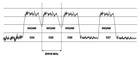
Figure 21. Example of digital channels spectrum.
