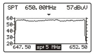
Figure 39. SPECT mode, span reduction.
