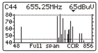
Figure 11. SCAN mode with reference line at 45 dBµV.
