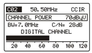
Figure 19. Measuring a digital channel.
