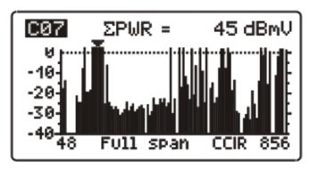
Figure 12. SCAN mode, power detection function.
