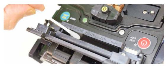
Figure 34. Clean the Heating Plate.
