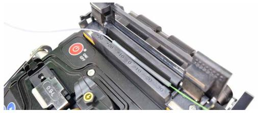
Figure 26. Place Fibre with Protection Sleeve.
