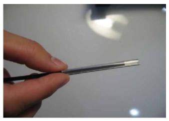
Figure 13. Placing Protection Sleeve.
