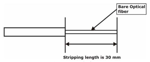
Figure 14. Stripping Length of Coating Layer.
