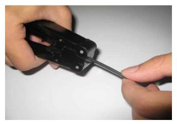
Figure 11. Butterflied Fibre Strip.
