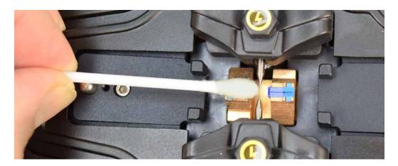
Figure 29. Clean The Electrodes.
