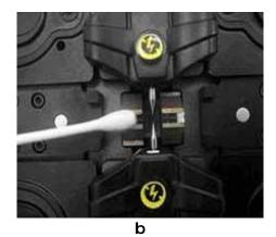
Figure 31. Clean the V-groove.
