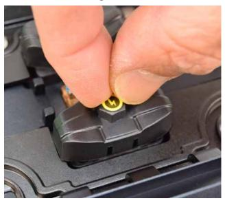
Figure 30. Electrodes-replace.
