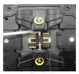
Figure 32. Clean the Microscope.
