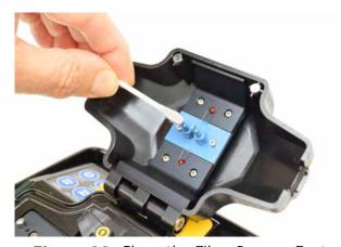
Figure 33. Clean the Fibre Presser Foot.
