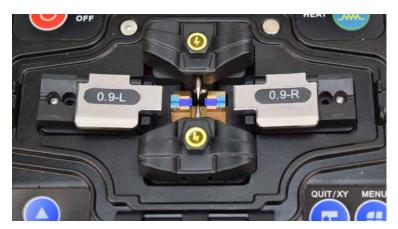
Figure 17. Fibre-Place.
