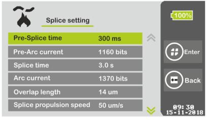
Figure 20. Splice Parameters Menu (a).
