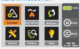
Function: Set the parameters of some system functions such as heating
