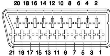
**Figure 28.-** Scart socket (external view).
