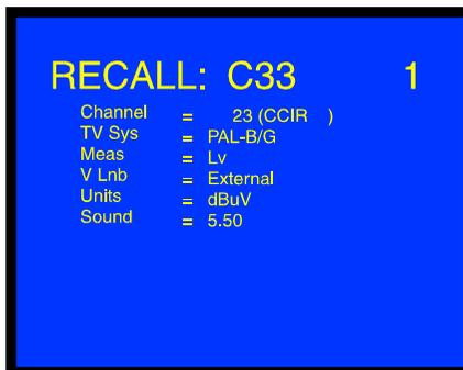
**Figure 22** .- RECALL screen, retrieving a measurement configuration.
