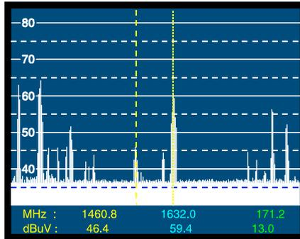
Figure 18.- Spectrum Analyser mode with two tuning markers.
