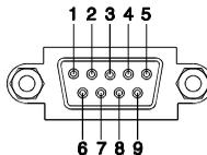
**Figure 24.-** Connector RS-232C **PROLINK-3**. Pins numbering.
