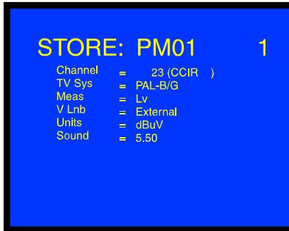
**Figure 21** .- STORE screen, storing a measuring configuration.
