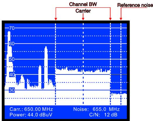
**Figure 19.**-Carrier to Noise measurement in Spectrum mode (digital channel).
