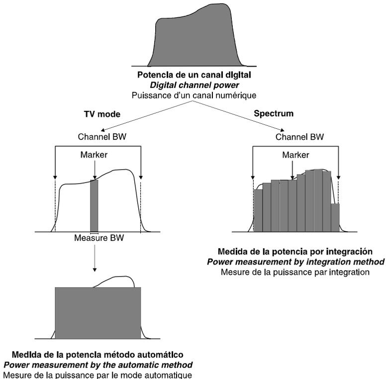
**Figure 9.-** Measuring digital power.
