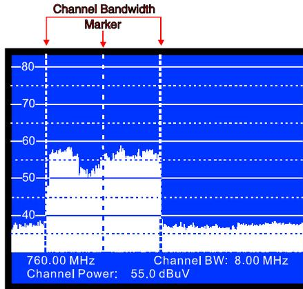
Figure 20.- Channel power measurement in Spectrum Mode.
