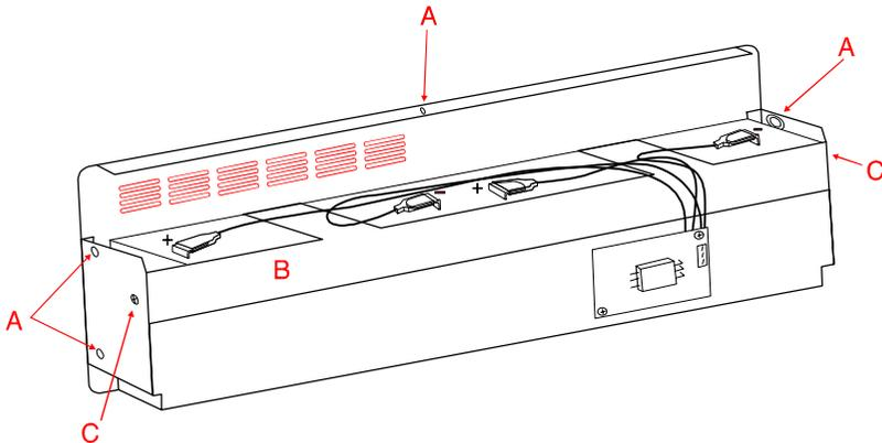
Figure 29.- Battery compartment.
