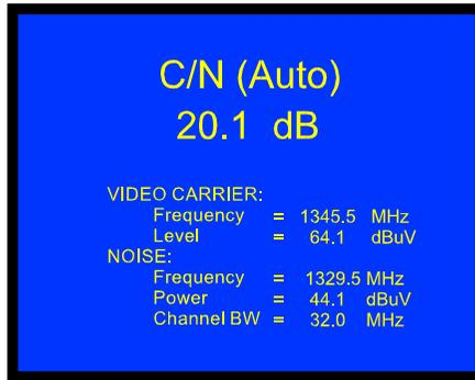
**Figure 8.-** Carrier-to-noise ratio measurement (Satellite band, analogue signal).
