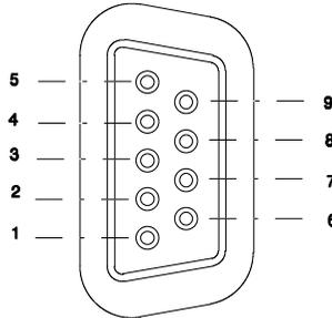
**Figure 27.-** RS-232C connector. External view.
