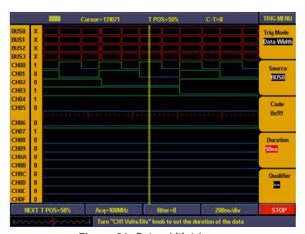
Figure 86. Data width trigger.
