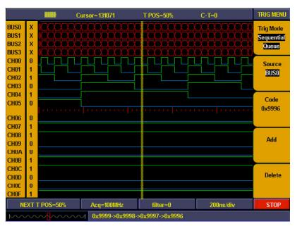
Figure 82. Sequential queue trigger.
