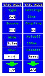
Figure 45. Alternate trigger (Trigger Type: Pulse) Menu.
