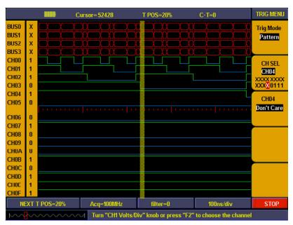
Figure 80. Pattern trigger menu.
