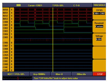
Figure 88. Threshold setting menu.
