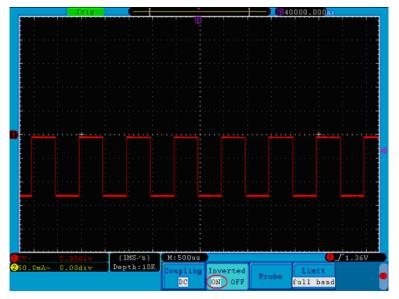
Figure 21. Inverted Waveform.
