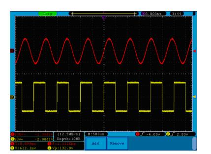
Figure 65. Automatic measurement.
