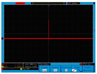
Figure 84. Capturing a Single Signal.
