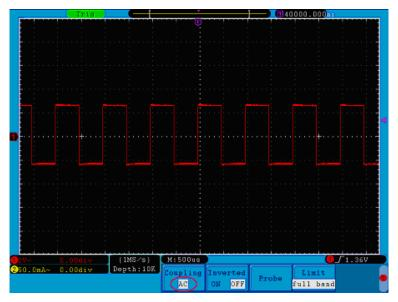
Figure 17. AC Coupling Oscillogram.
