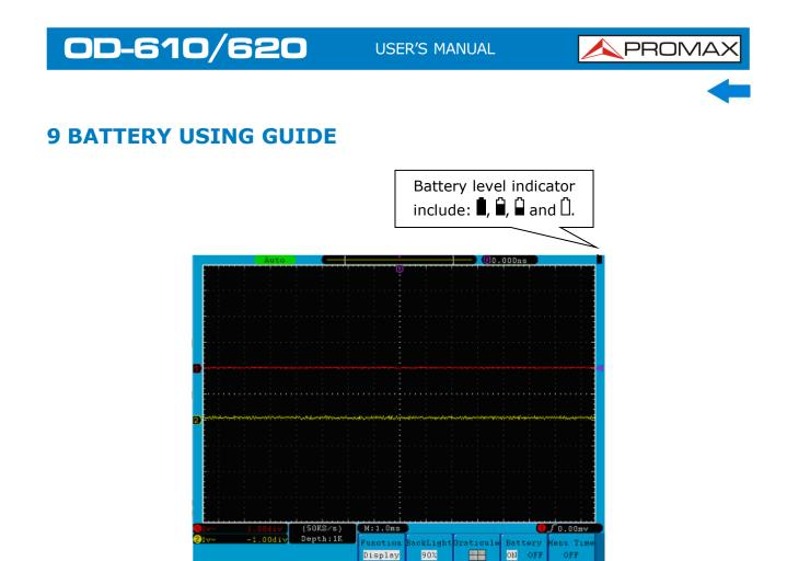
Figure 89. Battery level indicator.
