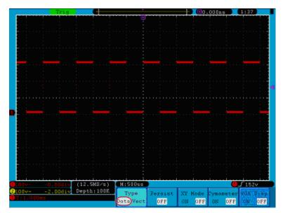
Figure 47. Display in Dots form.
