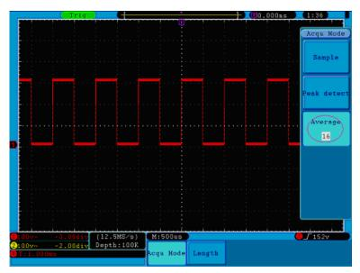
Figure 86. Reduce Noise level by using Average function.
