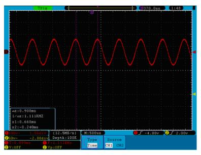
Figure 70. Waveform of Cursor Measurement.
