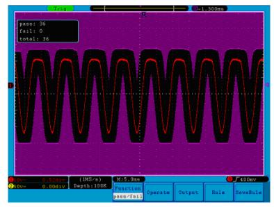
Figure 61. Pass/Fail test
