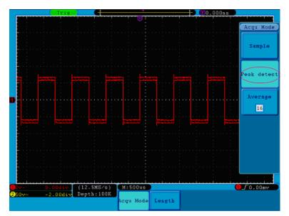
Figure 85. Signal with Noises.
