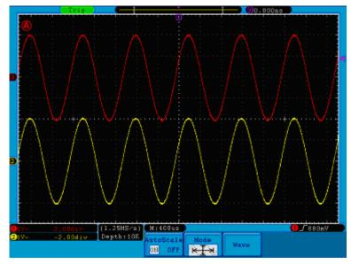
Figure 75. Autoscale Horizontal-Vertical multi-period waveforms.
