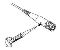
Figure 9. Adjust Probe.
