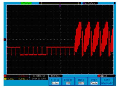
Figure 88. Waveform Captured from Video Field Trigger.
