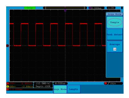
Figure 43. Normal ACQU Mode display, in which no burr can be detected.
