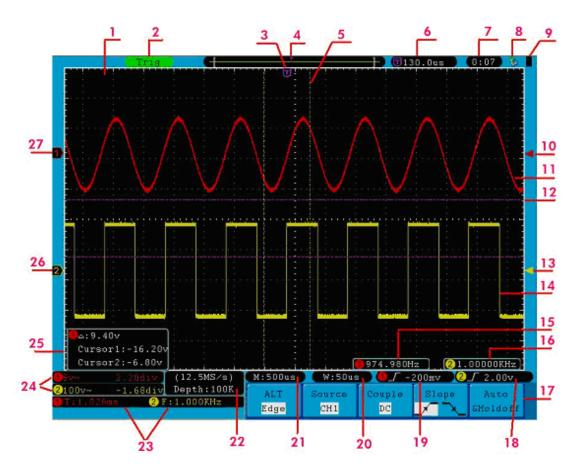
Figure 6. Illustrative Drawing of Display Interfaces.
