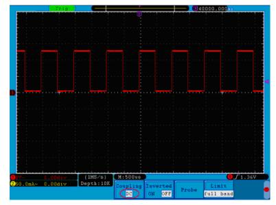
Figure 16. DC Coupling Oscillogram.
