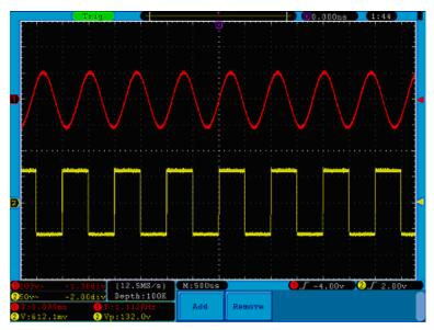
**Figure 82.** Measure Frequency and PK-PK value for a given signal.
