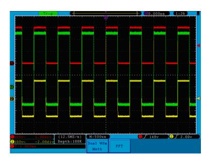
Figure 23. Waveform resulted from CH1 +CH2.
