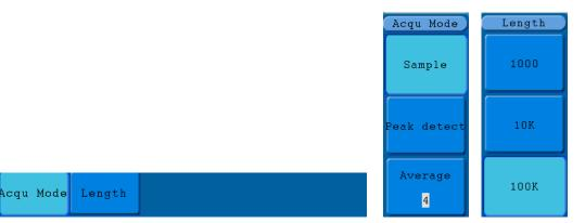
Figure 38. ACQU MODE Menu (OD-603 does not have "Length" menu).
