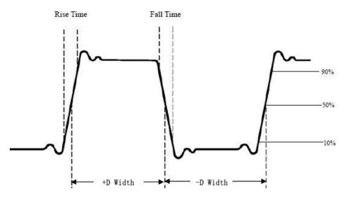
Figure 64. Shows a pulse with some of the time measurement points.
