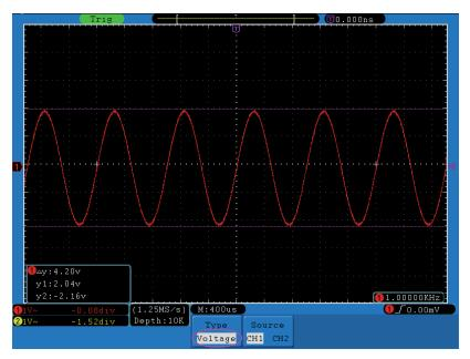
Figure 66. Waveform of Voltage Cursor Measurement.
