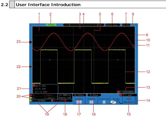
Figure 5. Illustrative Drawing of Display Interfaces (take OD-603) for instance)
