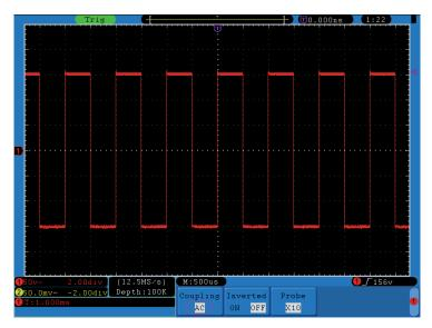
Figure 15. AC Coupling Oscillogram.
