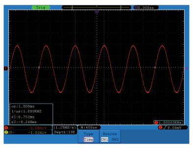
Figure 67. Waveform of Cursor Measurement.
