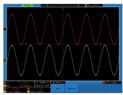
Figure 62. Automatic measurement.
