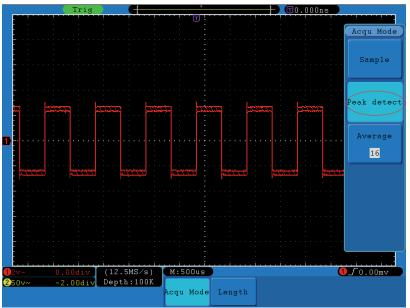
Figure 83. Signal with Noises.
