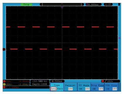
Figure 44. Display in Dots form.
