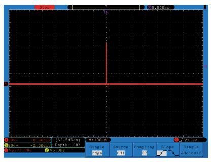
Figure 82. Capturing a Single Signal.
