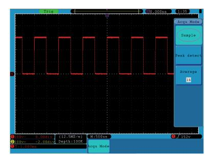
Figure 40. Normal ACQU Mode display, in which no burr can be detected.
