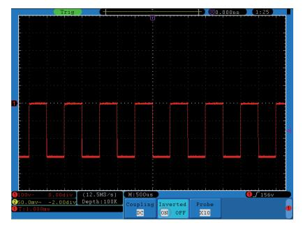
Figure 18. Inverted Waveform.
