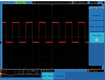
Figure 84. Reduce Noise level by using Average function.
