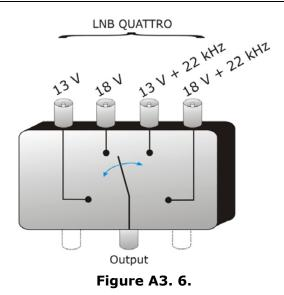
In the **DiSEqC<sup>TM</sup>** menu of the HD **RANGER**, select the band and the polarisations desired and send the SAT A command, as it is indicated in the following table:
