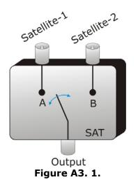
It is the simpler **DiSEqC<sup>™</sup>** switcher. This one uses the « SAT A/B » commands and allows to switch between two different Universal LNB:
