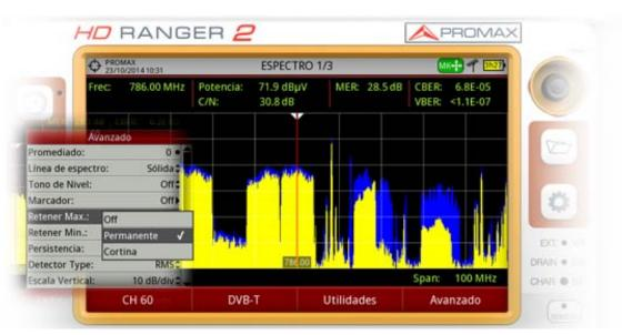
Figure A7.4 Max hold on the signal. The maximum power of the spectrum is traced in blue, behind the real-time spectrum (yellow).
