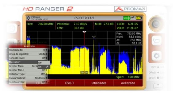
Figure A7.5 Marker enabled and placed in one of the LTE channels, at the frequency 793.5 MHz.
