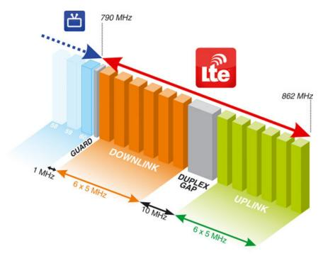
Figure A7.2 Picture of the terrestrial band occupied by LTE frequencies.
