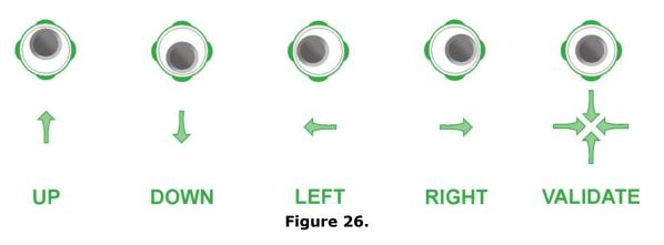
The joystick is multifunctional, that is, each time you press its function changes. The user can see the active function according to the icon that is displayed at the upper right corner of the equipment, as shown in the image.
