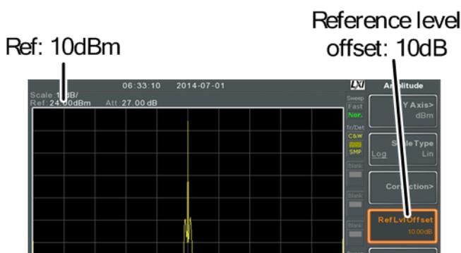
Figure 29. After reference level offset (offset: 10dB)
