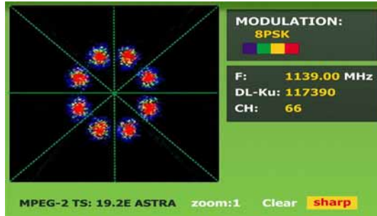
Figure 49.- Constellation Diagram. DVB-S2 (8PSK) signal.
