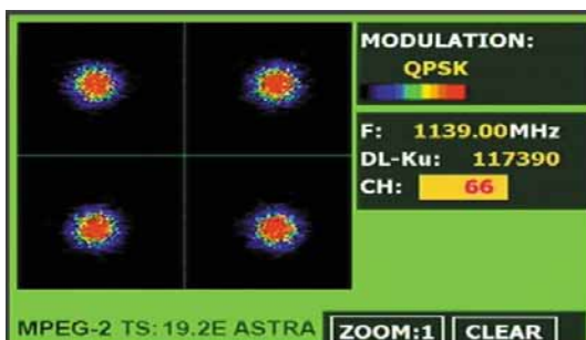
Figure 48.- Constellation Diagram. DVB-S (QPSK) signal.
