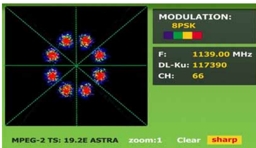
Figure 49.- Diagramme de constellation. Signal DVB-S2 (8PSK).
