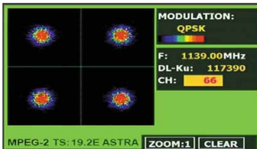
Figure 48.- Diagramme de constellation. Signal DVB-S (QPSK).
