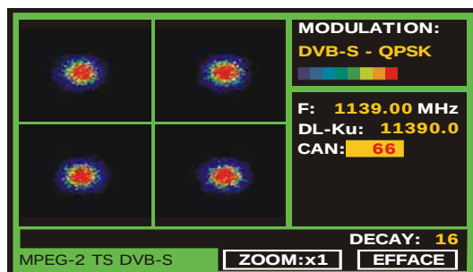
Figure 44.- Diagramme de constellation. Signal DVB-S (QPSK).
