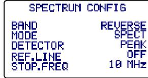
Figure 33.- SPECT mode configuration.
