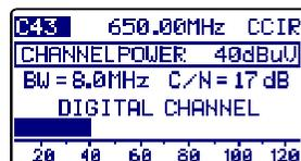
Figure 17.- Measuring a digital channel.
