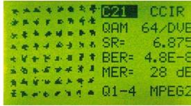
**Figure 20.-** Constellation Diagram representation and BER and MER measurement in a digital channel.
