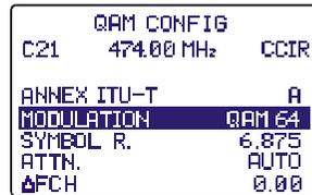
**Figure 21.-** Configuration of digital signal measurement.
