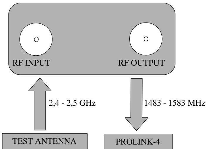
First of all the RF output should be connected to the spectrum analyser input using the supplied coaxial cable. The signal source or the test antenna should then be connected to the down converter RF input to finally activate the spectrum analyser power supply. If the CV-245 is used with PROLINK-2+, PROLINK-3/3C *Premium* or PROLINK-4/4C *Premium* spectrum analysers the drain indication on the analyser will confirm that the down converter is active.
