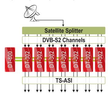
Thanks to the CAM interface available in the DT-302's it is also possible to decrypt the **HDTV** channels right at the headend.
