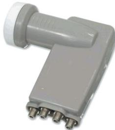
A **Quattro-LNB** is a LNB with 4 outputs that provides in a separated way the four frequency bands (vertical low, vertical high, horizontal low and horizontal high). These four signals can then be distributed in the building through multiswitches.
