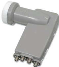
A **Quattro-LNB** is a LNB with 4 outputs that provides in a separated way the four frequency bands (vertical low, vertical high, horizontal low and horizontal high). These four signals can then be distributed in the building through multiswitches.
