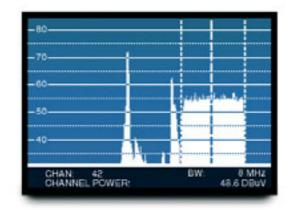
multiplex in the adjacent channel. To solve this, the digital multiplex can be shifted forward.
