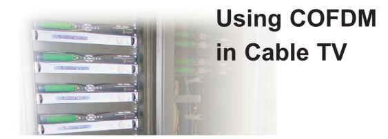
Cable TV networks are going through a process of digitalisation of their services and are facing important investments. PROMAX proposes the use of COFDM modulation scheme instead of usual QAM modulators. This method allows a much easier access to the subscribers with implementation costs that can be dramatically reduced. In addition the system is more robust.
