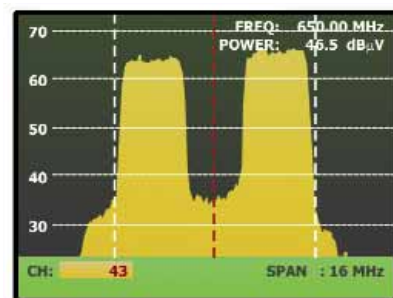
Spectrum hole unveiling the presence of intermodulation products within the channel
