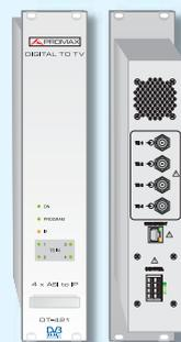
The **DT-421** IP Streamer module can receive multiple ASI Transport Streams and delivers an IP-encapsulated stream for distribution over the Ethernet Network.
