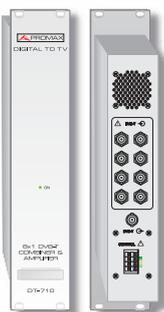
**DT-710** is an eight inputs and one output combiner designed to add the output multiplex generated by the **Digital To TV** to the existing DTT channels in the area. It provides a 114 dB $\mu$ V (+6 dBm) output signal, which is quite usual for SMATV systems. The **DT-722** provides a 130 dB $\mu$ V (+22 dBm) output.
