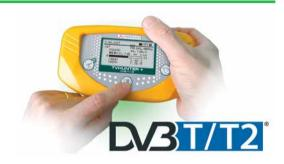
The meter shows information about the received signal power (wide band analogue and digital) in the form of two graphic bars with two different time constants and an audible indicator to help align the aerial to the optimum detection.
