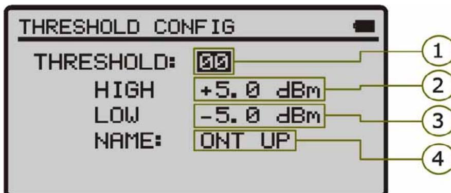
Figure 6. Écran THRESHOLD CONFIG.
