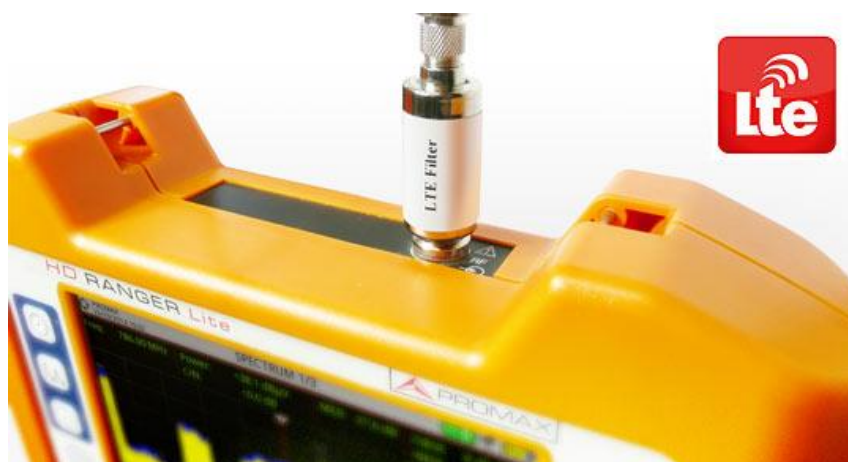
Figure A8.6 LTE filter coupled to a HD RANGER Lite field strength meter.
