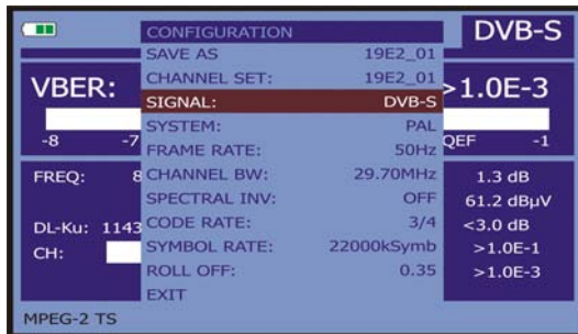
Figure 21.- Measurement configuration screen ( QPSK signals).
