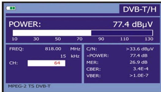
Figure 28.- Digital channel power measurement.
