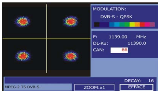
Figure 44.- Diagramme de constellation. Signal DVB-S (QPSK).
