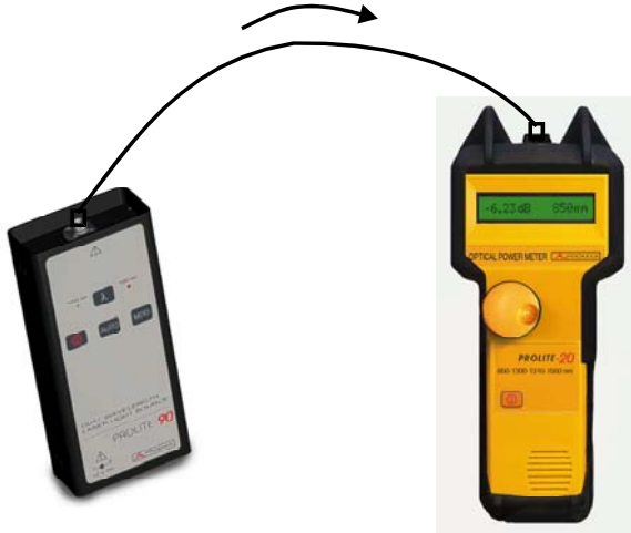
Figure 2. – Measuring the reference power
