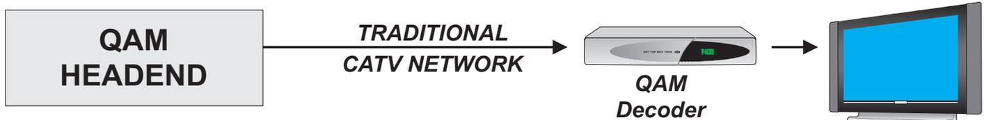
*Standard digital CATV network configuration: Expensive headend QAM modulators and subscriber extra cost due to all the QAM decoders must be rented or bought*
